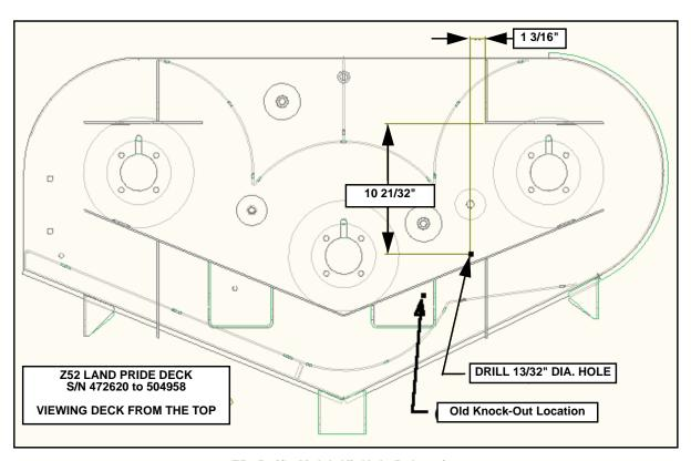
Z52 Baffle Mulch Kit Hole Relocation Figure 2
